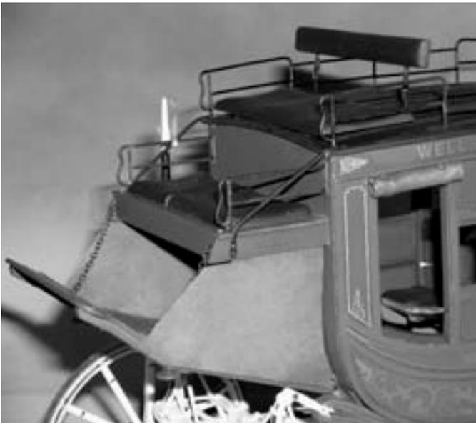
Photo 28: Front boot detail, roof top passenger seat
