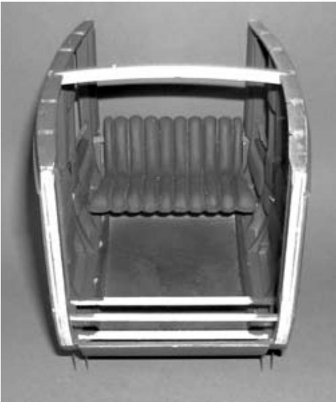
Photo 22: Seat supports and seat installation
