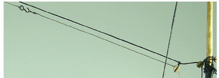
main mast. Be sure to run the halliard through the lubber's hole of the main top first. Finish it off with a rope coil.
