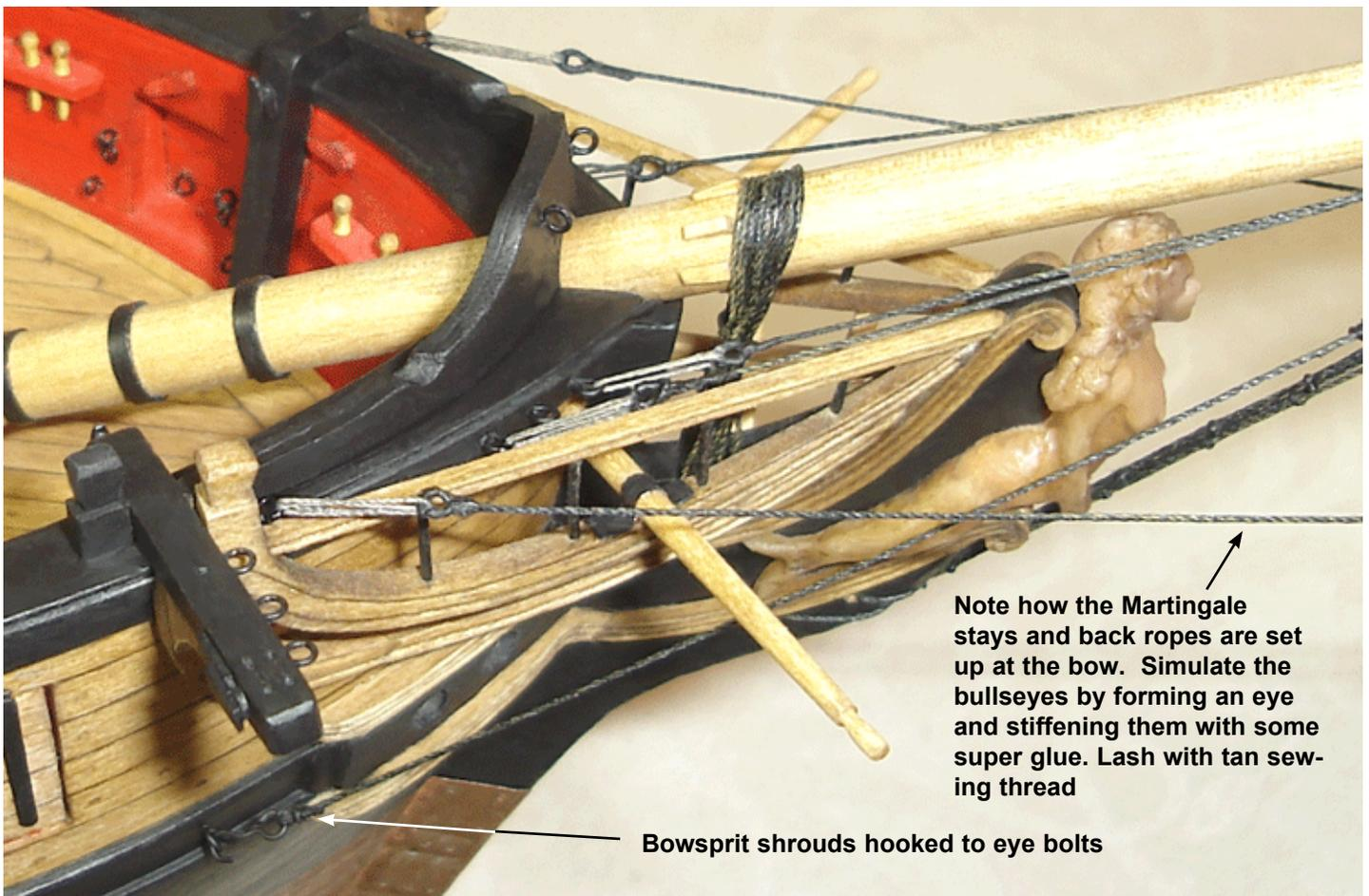
Note how the Martingale stays and back ropes are set up at the bow. Simulate the bullseyes by forming an eye and stiffening them with some super glue. Lash with tan sewing thread
