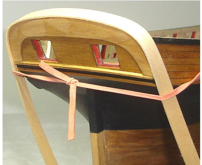
strips may be a little heavy and should be thinned down a little bit with the edges rounded off.  $1/32'' \times 1/32''$  is probably too thin, but something in between would work fine. The area between the two molding strips should be no less than  $1/8''$  wide. Be sure to follow the gentle curve of the transom side-to-side and keep the space between them consistent.
