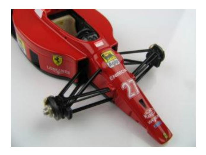
Drive shafts, brake ducts and brake disks can then be added. It is important to check the fit of each component at this point and where necessary, re-drill attachment points to clear paint build-up. Also consider the sequence of the build up to ensure all parts can be easily handled.
