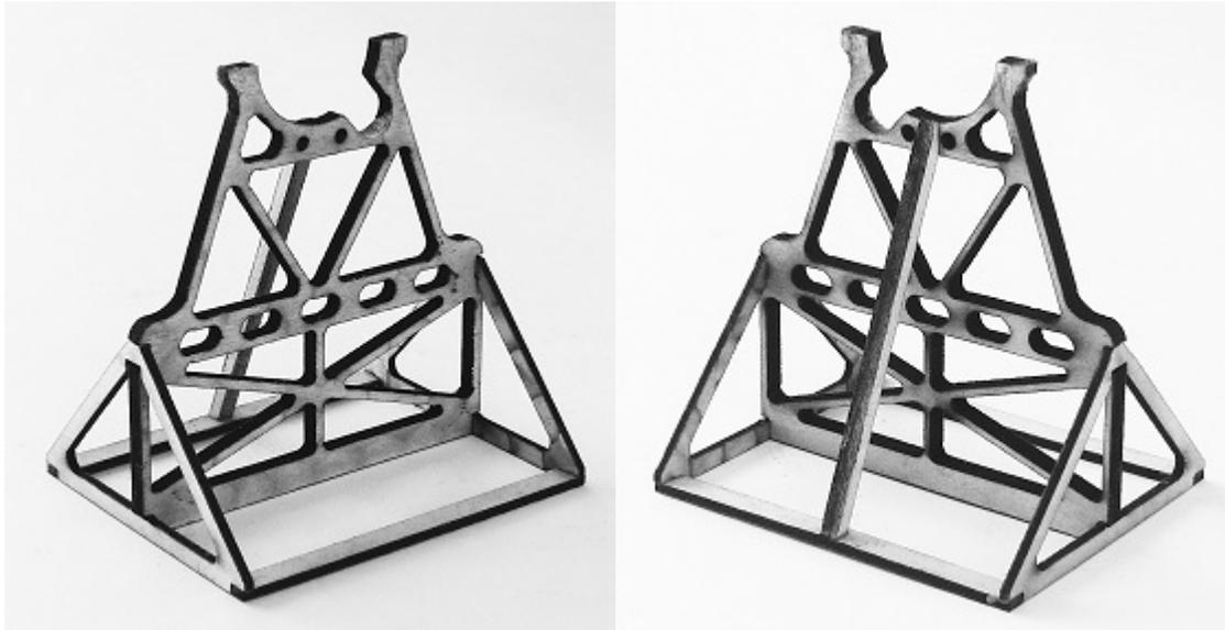
Using wood glue, assemble six of the seven laser-cut parts per the photographs, taking care that the base is square. Angle brace CLE908c is centered between the two small holes below the engine cradle in part CLE908a. Semicircular piece CLE908b is attached later. The actual stand would be steel, so primer coat the assembled stand and paint your desired color. Note the orientation of parts CLE916b.
