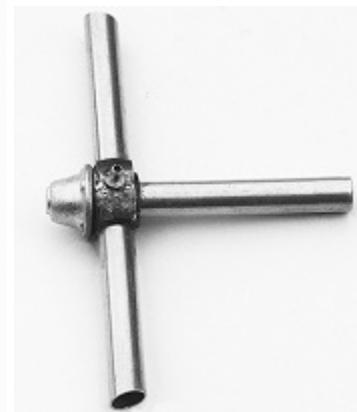
Glue the gear housing assembly to the engine stand. The stand cradle should snug up against the flange on the gear housing.
