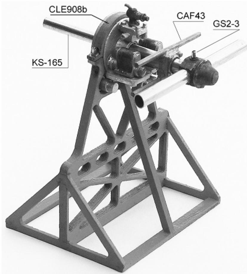
The rear engine support (CAF43) is optional in this arrangement, though it does help to balance the weight of the completed model, and is therefore recommended. Should you wish to use it, paint it zinc chromate green and slide it onto the brass tube. Do not glue yet.
