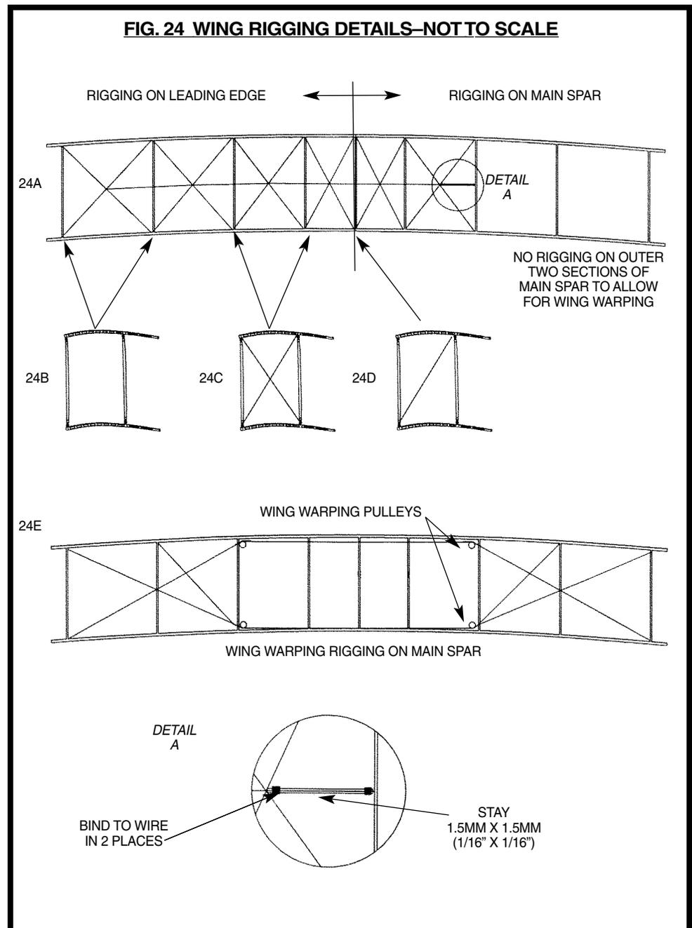
rigging is completed the center section of the structure will be rigid and the trailing edge of the tips will be free to flex up and down to control the aircraft's roll. This wing warping was patented by the Wrights.
