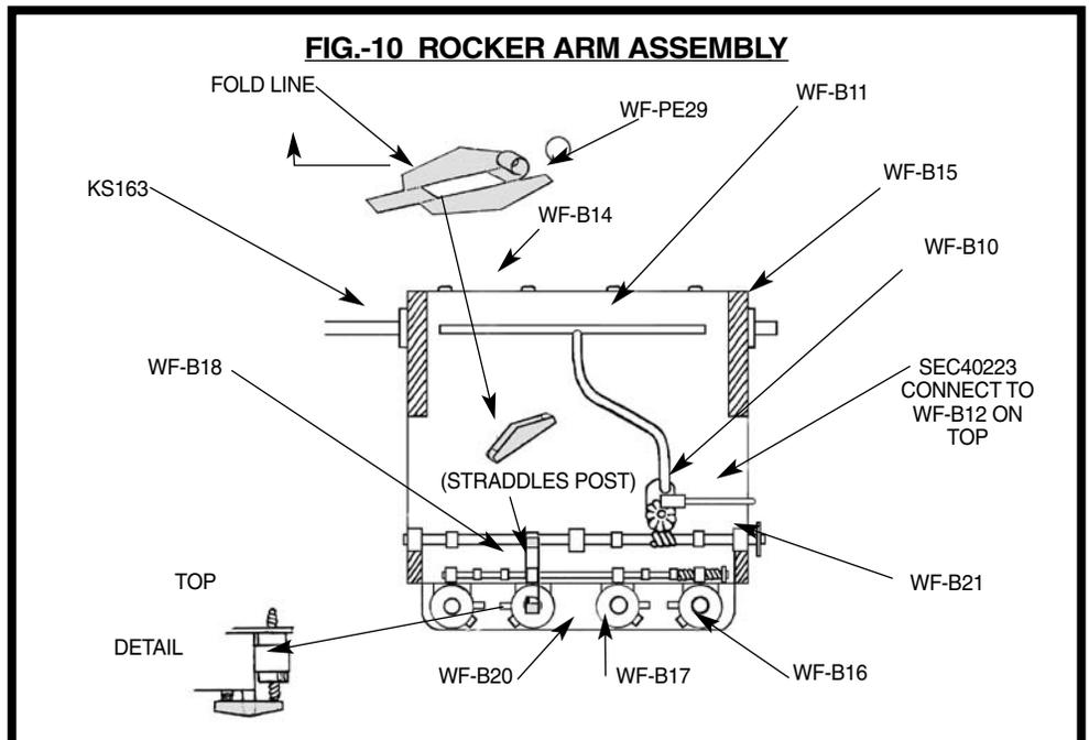
fits into the hole in the oil pump. Bend and glue in place the four exhaust rocker arms (WF-PE29). Roll the tabs inward
