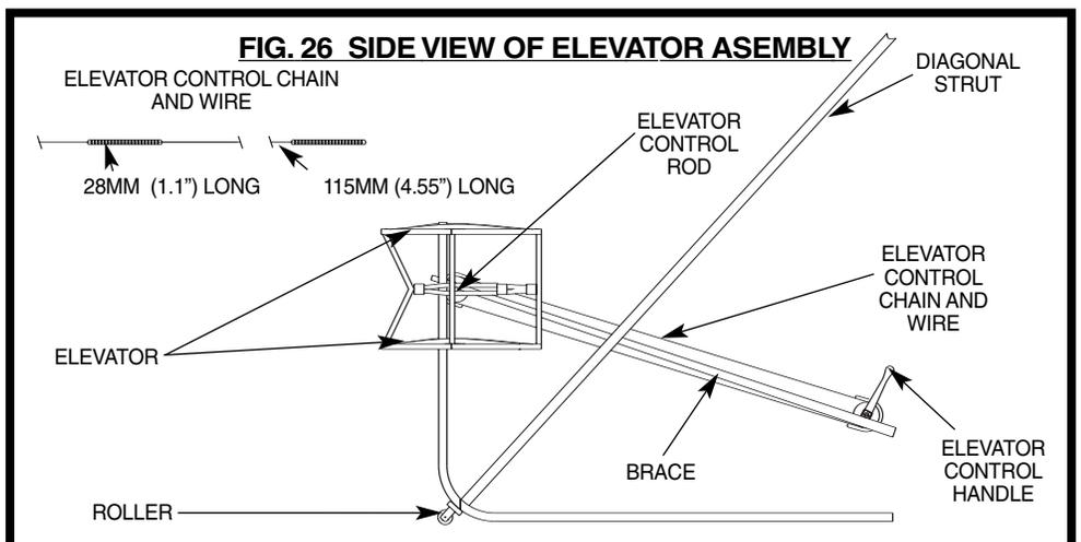
glue WF-L16 to WF-L17 for the two sides of the elevator control frame. Add the diagonal strut flush with inside of frame. Taper brace from 1.5 x re. Add brace to inside surface of diagonal strut and frame. Glue to diagonal strut, but **DO NOT GLUE BRACE TO FRAME** or you will not be able to get the elevators on.
