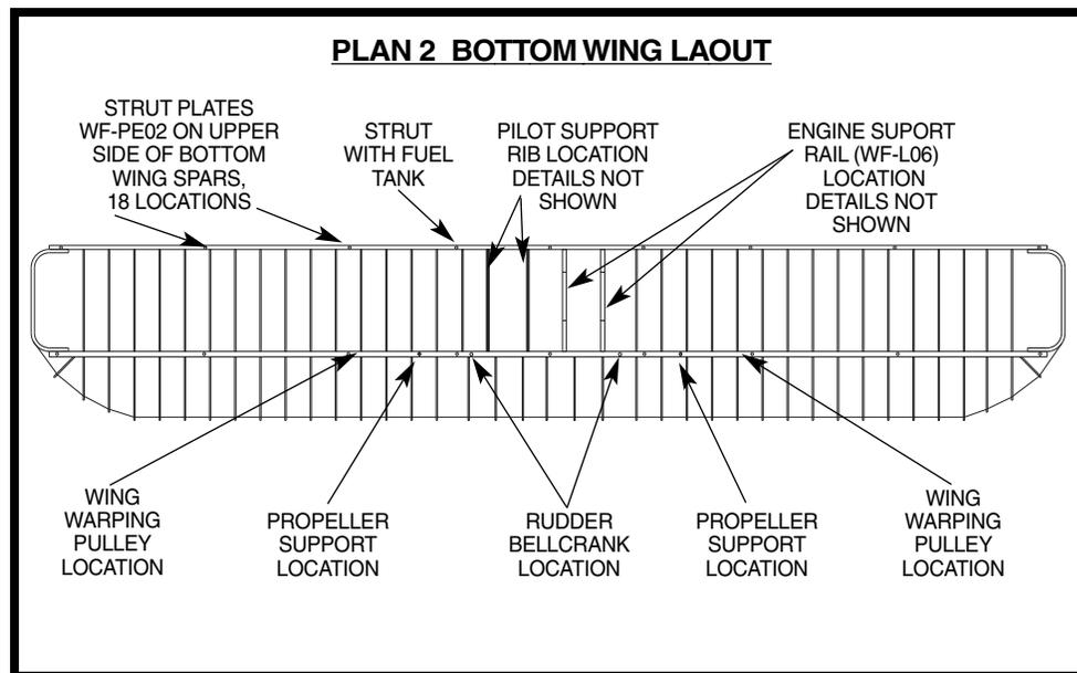
Before assembling the bottom wing drill holes in the top of the main spar for the propeller support assembly WF-B30 as described in the instructions for the top wing. Additionally drill .75mm (.031" (#68)) hole for rudder bell cranks at the two locations shown on Plan 2. Do not go all the way through the spar.
