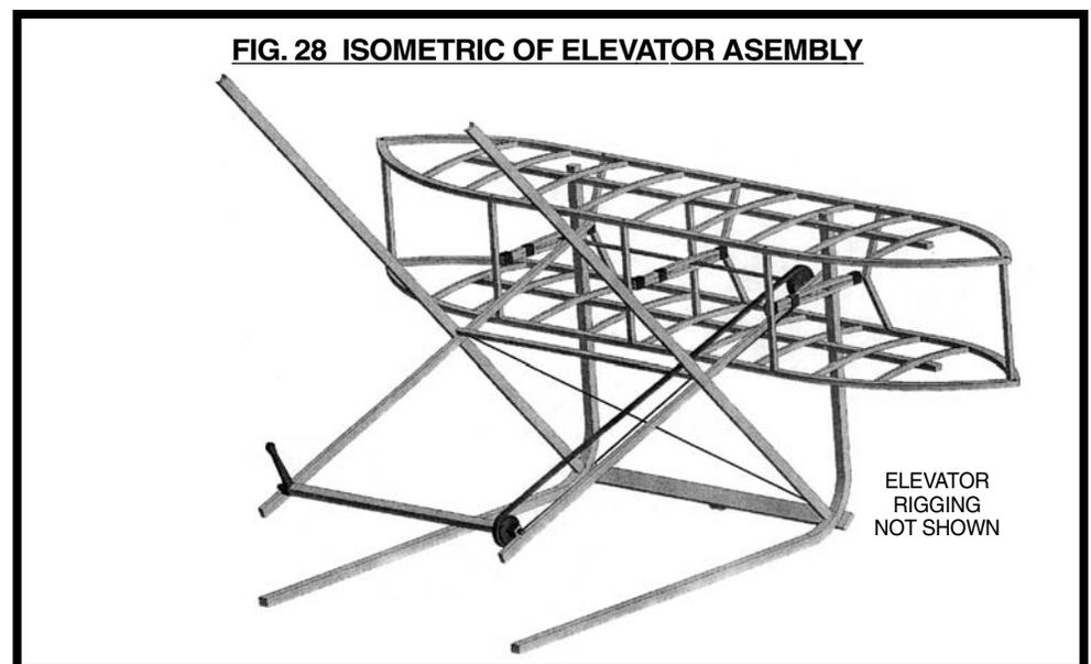
in Figure 29 is completed it should be mounted on the elevator control frame. Either the center spar is glued to the outrigger or, if motion is desired, short lengths of thread are used as hinges.
