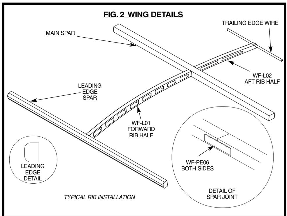
and bottom edges as shown in Figure 2. Carefully taper the leading edge spar from last rib to the tip at both ends. The taper should be the same on both top and bottom of the spar and tip thickness should match the thickness of the laser cut wing tip 3mm (1/8"). The main spar needs no taper.
