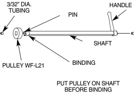
**FIG. 32 ELEVATOR ASSEMBLY CONNECTION**
