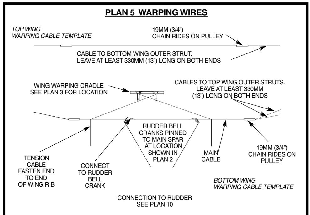
Install the rudder bellcranks (WF-PE01) at the locations shown on Plan 2. Attach to the wing warping wire with short lengths of thread as shown. As with the wing warping wires temporarily secure the ends that go to the rudder.
