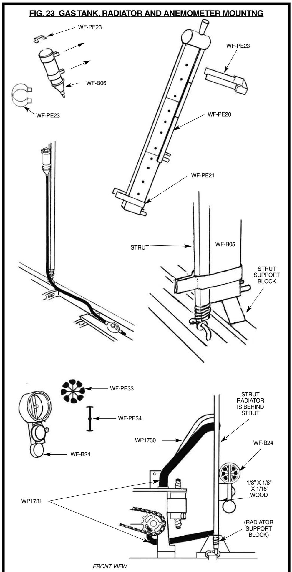
to conform to this. The procedure for the bottom strap (WF-PE21) is similar but without the step bends. Glue the bottom strap to the radiator, just above the plug above the bottom nipple. Glue the top strap just under the top rivet.
